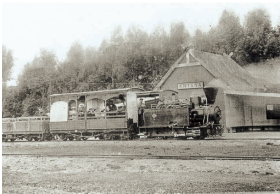
An early Orenstein & Köppel 'coffee-pot' locomotive and passenger coach of the South-Western Railway Company departing from a station near Knysna Knysna Museum
