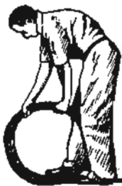
PROPER METHOD OF UNCOILING WIRE ROPE.
