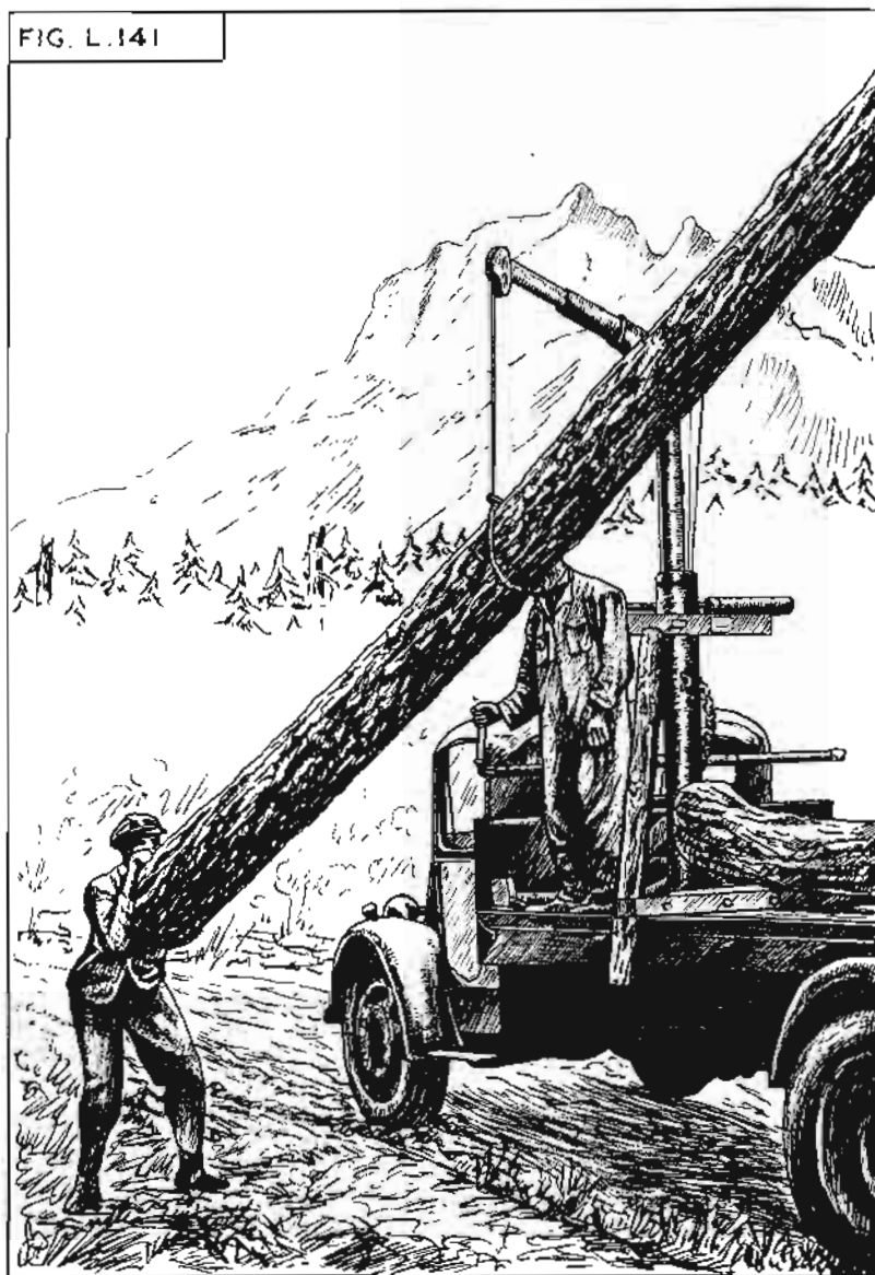
HEAVY, LONG LOGS UP TO 0.5 TONS CAN BE LOADED SINGLY BY SELF-LOADING LORRIES. HERE THE ASSISTANT IS PRESSING DOWN ON THE BUTT WHILST OPERATOR LIFTS AND TRAVERSES
