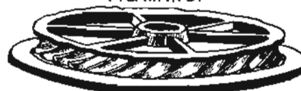
SHEAVE WITH CORRUGATED GROOVE AND FLANGE WORN OFF BY ROPE.
