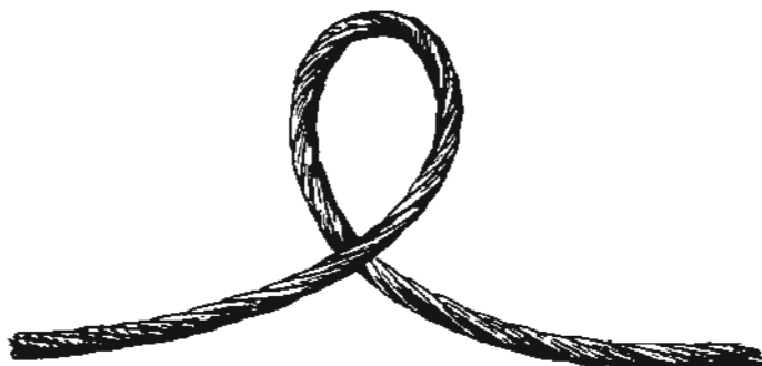
CABLE IN POSITION TO KINK.
