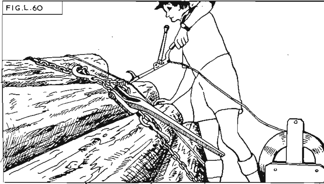
APPLYING STRAPPING TO A STACK OF LOGS PRETIGHTENED WITH A CHAIN AND TOGGALOCK.
