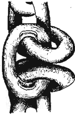
CHAIN SHOWING INTERLINK WEAR.
