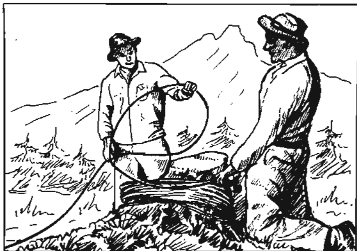
UNWINDING ROPE COILED AROUND STUMP CAN PRODUCE KINKS.
