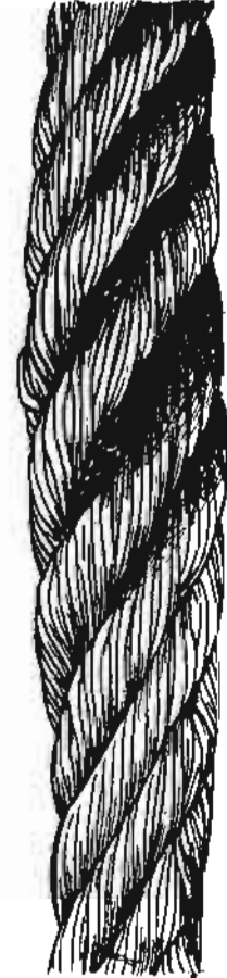
DAMAGED BY BAD SHEAVE GROOVES. DAMAGED BY HEAVY LOADS ON SMALL, SMOOTH DRUMS.
