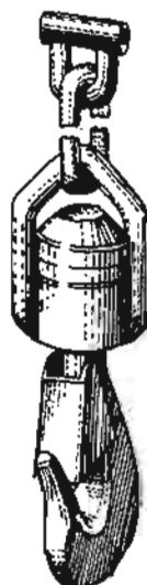
JIB-ATTACHED SWIVEL LOADING HOOK.
