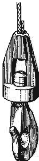
LOADING SWIVEL LINE HOOK WITH SAFETY CATCH.
