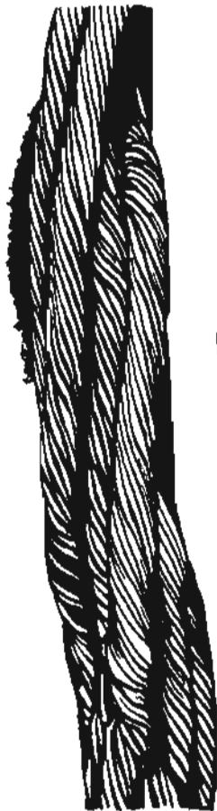
ROPE DAMAGED BY KINKING.
