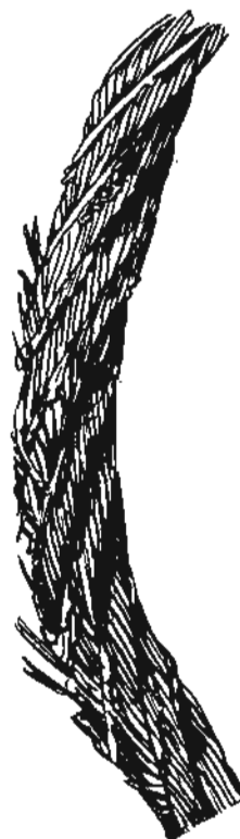
EXCESSIVE BENDING AROUND SMALL SHEAVES.
