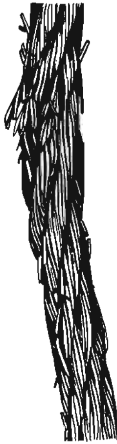
ROPE DAMAGED BY KINKING.
